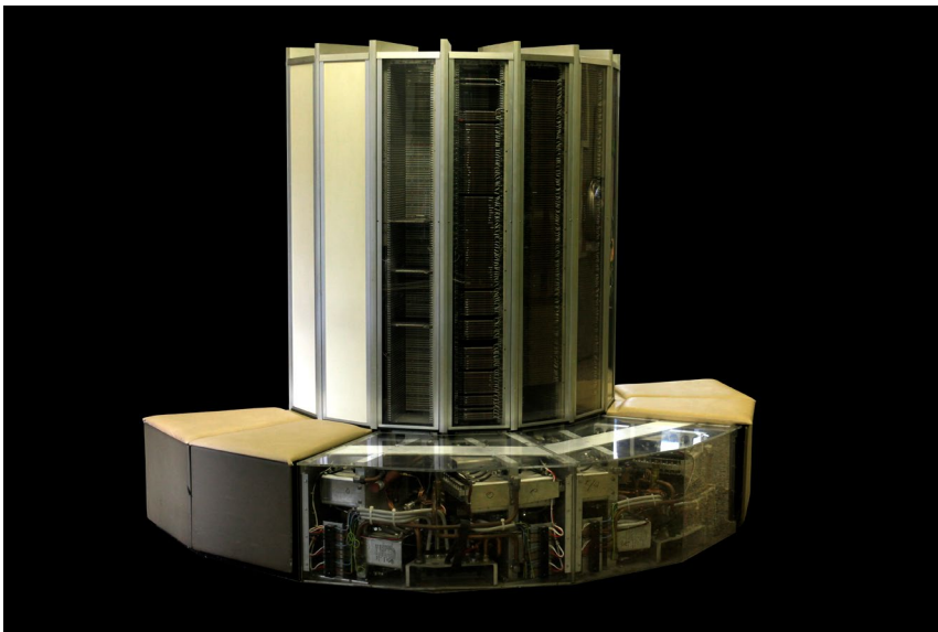
Cray-1 from 1976. Instead of aesthetics, the eccentric design is based on the optimisation of component distances and heat transfer.
